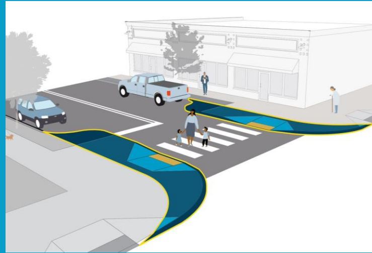
Curb extensions on side streets
